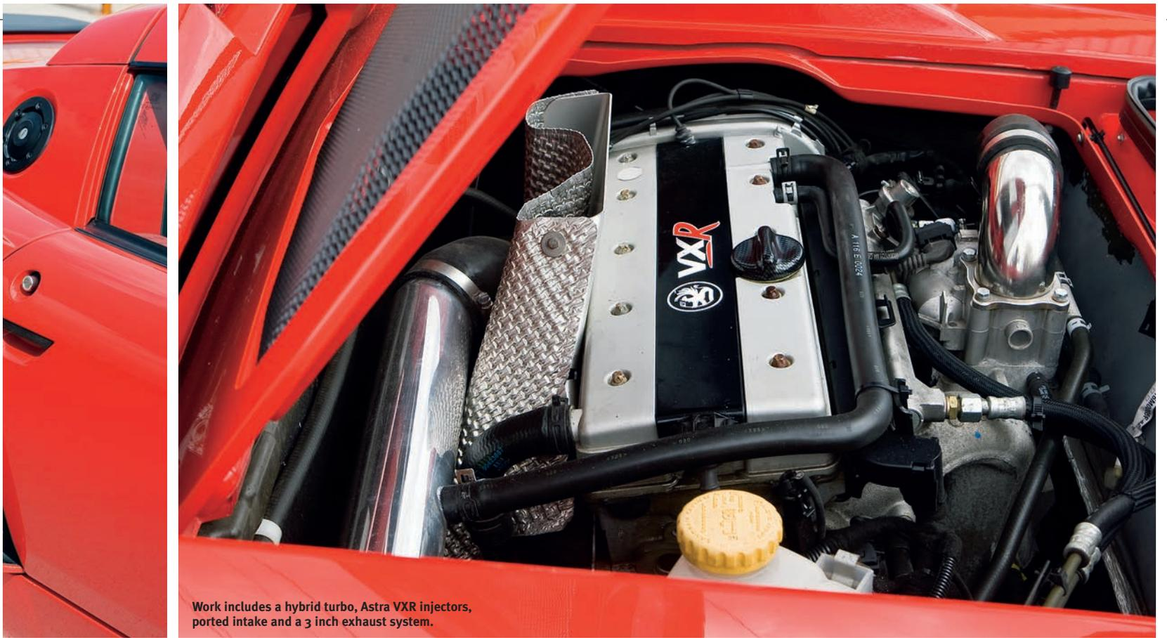
Work includes a hybrid turbo, Astra VXR injectors, ported intake and a 3 inch exhaust system.
